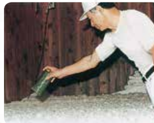
The toji (the chief sake maker) scatters koji spores onto rice in a koji -making room at a temperature approximately 30°C.
