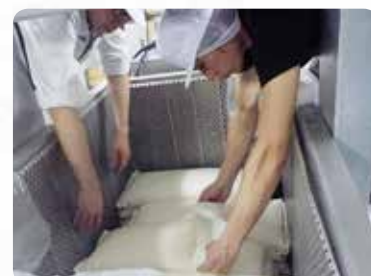
The mash is poured into bags, and the bags are laid in a traditional press
