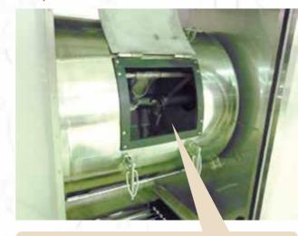
Rice is washed in this rotating drum. On the next day, rice is steamed and the koji making process takes place inside the drum under controlled temperature.
